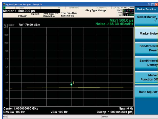
Figure 5b. An MXA shows -165.38 dBm DANL normalized to RBW of 1 Hz, with the preamplifier on.
