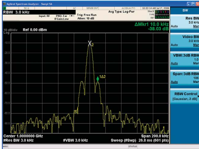
Figure 6a. Testing a 2.5% depth AM signal with an MXA (RBW=VBW=3 kHz), the AM sideband can be clearly seen (at Marker 1Δ2).
