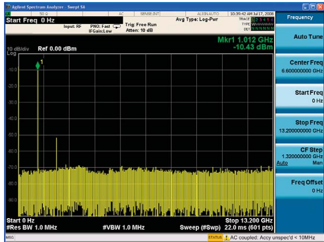
Figure 4b. The MXA only takes 22 ms for a full span of 13.2 GHz sweep (RBW=VBW=1 MHz).
