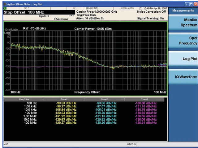
Figure 10b. Phase noise log plot obtained with N9068A phase noise measurement application in an MXA—much faster and easier to use than the 85671A.
